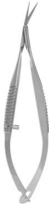
Vannas Scissors 13-078 Sharp tips. Angled to side 7mm blades, 9mm from pivot to tip, 8 cm long
